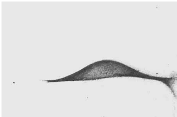
Fig. 8. Two dimensional immunoelectrophoresis of a pure alkaline phosphatase preparation (Sample 110 \mu\text{g} ; electrophoresis: first direction (anode left), 40 min at 250 V in 0.8% agarose, pH 8.6; second direction (anode above) 15 h at 100 V in antiserum containing agarose (2 ml of rabbit antiserum + 38 ml of 0.8% agarose) in Na-barbital buffer, 0.1M, pH 8.6; Stain: Amidoschwarz 10B )
